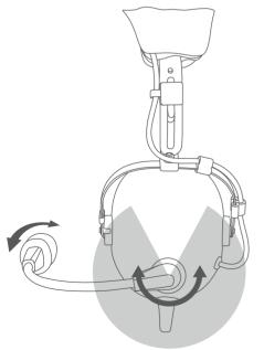
To adjust the microphone placement, rotate the microphone from its base and bend the flexible boom.
