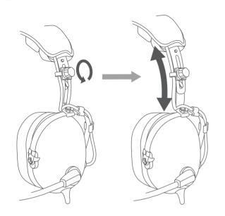
Adjustment for a personalized fit on the headset is simple and easy. Proper fit is important both for comfort and optimal noise reduction.
